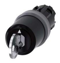
Key-operated switch IKON, 22 mm, round, plastic with metal front ring, lock number 360012K1, with 2 keys, 3 switch positions I-O-II, latching, actuating angle 2x45°, 10:30h/12h/13:30h, Key removal I+O+II, with laser labeling, upper case
