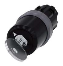
Key-operated switch BKS, 22 mm, round, plastic with metal front ring, special lock, with 2 keys, 2 switch positions O-I, latching, actuating angle 90°, 10:30h/13:30h, key removal O+I, Note: BKS locking systems E1 - E25 supplied without key
