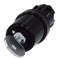
Key-operated switch BKS, 22 mm, round, plastic, lock number S1, with 2 keys, 2 switch positions O-I, latching, actuating angle 90°, 10:30h/13:30h, key removal I, with laser labeling, upper case and lower case, always upper case at the beginning of the word
