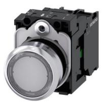
Illuminated pushbutton, 22 mm, round, metal, shiny, clear, pushbutton, flat, momentary contact type, with holder, 1NO, LED module with integrated LED 110 V AC, screw terminal, with laser labeling, upper case
