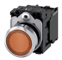
Illuminated pushbutton, 22 mm, round, metal, shiny, amber, pushbutton, flat, momentary contact type, with holder, 1NO, LED module with integrated LED 24 V AC/DC, screw terminal, with laser labeling, upper case
