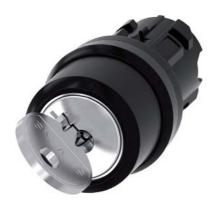
RONIS key-operated switch, 22 mm, round, plastic, lock number SB30, with 2 keys, 2 switch positions O<I, momentary contact type, Actuating angle 45°, 10:30h/12h, key removal O, possible special locks: SB31, 421, 455 Z=50-unit packaging
