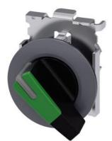
Selector switch, illuminable, 30 mm, round, Metal, matte, green, selector switch, long, front ring for flush installation, 2 switch positions O<I, momentary contact type, Actuating angle 45°, 10:30h/12h, Z=50-unit packaging
