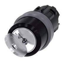
RONIS key-operated switch, 22 mm, round, plastic with metal front ring, lock number SB30, with 2 keys, 2 switch positions O-I, latching, actuating angle  $90^{\circ}$ , 10:30h/13:30h, key removal O+I, possible special locks: SB31, 421, 455, with laser labeling, lower case
