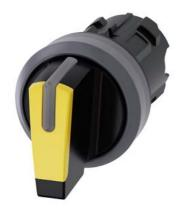
Selector switch, illuminable, 22 mm, round, plastic with metal front ring, yellow, selector switch, short, 3 switch positions I>O<II, momentary contact on the left, latching on the right, actuating angle 2x45°, 10:30h/12h/13:30h, with laser labeling, lower case
