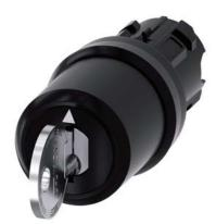
Key-operated switch IKON, 22 mm, round, plastic, lock number 360012K1, with 2 keys, 3 switch positions I-O-II, latching, actuating angle 2x45°, 10:30h/12h/13:30h, Key removal I+O+II, with laser labeling, upper case and lower case, always upper case at beginning of line
