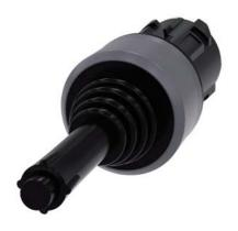
Coordinate switch, 22 mm, round, plastic with metal front ring, black, 4 switch positions, momentary contact type, with mechanical interlocking, with laser labeling, upper case and lower case, always upper case at the beginning of the word
