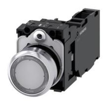
Illuminated pushbutton, 22 mm, round, Metal, shiny, clear, pushbutton, flat, momentary contact type, with holder, 1 NO+1 NC, LED module with integrated LED 230 V AC, screw terminal, with laser labeling, upper case
