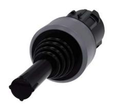
Coordinate switch, 22 mm, round, plastic with metal front ring, black, 2 switch positions, vertical latching, without mechanical interlocking, with laser labeling, upper case
