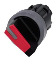
Selector switch, illuminable, 22 mm, round, plastic with metal front ring, red, selector switch, short, 2 switch positions O-I, latching, actuating angle 90°, 10:30h/13:30h, with laser labeling, upper case and lower case, always upper case at the beginning of the word
