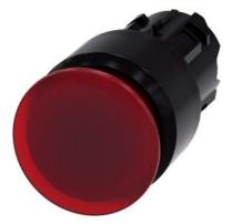
Illuminated mushroom pushbutton, 22 mm, round, plastic, red, 30 mm, latching, pull-to-unlatch mechanism, Z=50-unit packaging
