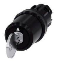
Key-operated switch BKS, 22 mm, round, plastic, lock number S1, with 2 keys, 3 switch positions I>O<II, momentary contact on the left, latching on the right, actuating angle 2x45°, 10:30h/12h/13:30h, key removal O, with laser labeling, inscription or symbol Customer-specific selection with SIRIUS ACT configurator (CIN)
