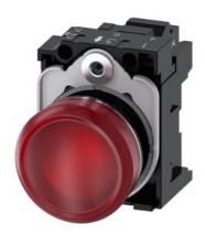
Indicator lights, 22 mm, round, metal, shiny, red, lens, smooth, with holder, LED module with integrated LED 110 V AC, spring-type terminal, with laser labeling, lower case
