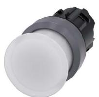
Illuminated mushroom pushbutton, 22 mm, round, plastic with metal front ring, white, 30 mm, momentary contact type, with laser labeling, symbol number according to, ISO 7000 or IEC 60417
