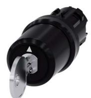
key-operated switch Siemens, 22 mm, round, plastic, lock number SSG10, with 2 keys, 3 switch positions I-O-II, latching, actuating angle 2x45°, 10:30h/12h/13:30h, key removal O, with laser labeling, upper case
