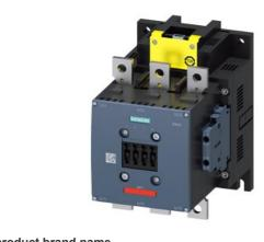
Power contactor, AC-3 225 A, 110 kW / 400 V Coil AC 50/60 Hz and DC 96-127 V x (0.8-1.1) F-SPS input 24 V DC 3-pole size S10 Auxiliary contacts 2 NO + 2 NC permanently mounted Main circuit: Busbar Control and auxiliary circuit: Screw terminal
