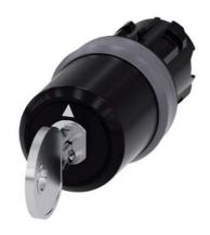
key-operated switch Siemens, 22 mm, round, plastic with metal front ring, lock number SSG10, with 2 keys, 3 switch positions I-O-II, latching, actuating angle 2x45°, 10:30h/12h/13:30h, key removal I, with laser labeling, upper case
