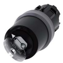
Key-operated switch IKON, 22 mm, round, plastic with metal front ring, special lock, with 2 keys, 2 switch positions O-I, latching, actuating angle 90°, 10:30h/13:30h, Key removal O+I
