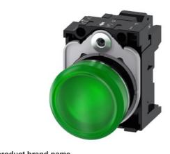
Indicator lights, 22 mm, round, metal, shiny, green, lens, smooth, with holder, LED module with integrated LED 110 V AC, spring-type terminal, with laser labeling, inscription or symbol Customer-specific selection with SIRIUS ACT configurator (CIN)
