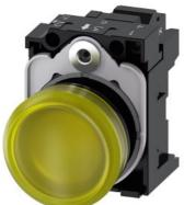
Indicator light, 22 mm, round, plastic, yellow, lens, smooth, with holder, LED module, with integrated LED 24 V AC/DC, spring-type terminal, with laser labeling, upper case and lower case, always upper case at beginning of line
