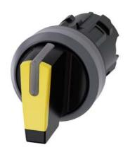
Selector switch, illuminable, 22 mm, round, plastic with metal front ring, yellow, selector switch, short, 3 switch positions I>O<II, momentary contact type, actuating angle 2x45°, 10:30h/12h/13:30h, with laser labeling, lower case
