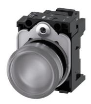
Indicator lights, 22 mm, round, metal, shiny, clear, lens, smooth, with holder, LED module with integrated LED 230 V AC, spring-type terminal, Z=20-unit packaging
