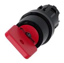
Key-operated switch O.M.R, 22 mm, round, plastic, lock number 73037, red, with 2 keys, 2 switch positions O<I, momentary contact type, Actuating angle 45°, 10:30h/12h, key removal O, with laser labeling, upper case and lower case, always upper case at beginning of line
