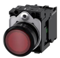
Illuminated pushbutton, 22 mm, round, plastic, red, pushbutton, flat, momentary contact type, with holder, 1NO, LED module with integrated LED 24 V AC/DC, screw terminal, with laser labeling, symbol number according to, ISO 7000 or IEC 60417
