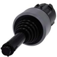
Coordinate switch, 22 mm, round, plastic with metal front ring, black, 2 switch positions, vertical, momentary contact type, with mechanical interlocking, with laser labeling, upper case and lower case, always upper case at the beginning of the word
