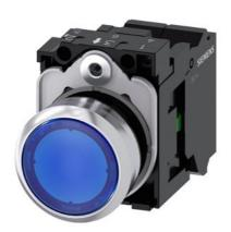
Illuminated pushbutton, 22 mm, round, metal, shiny, blue, pushbutton, flat, momentary contact type, with holder, 1NO, LED module with integrated LED 24 V AC/DC, spring-type terminal, with laser labeling, upper case
