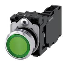
Illuminated pushbutton, 22 mm, round, metal, shiny, green, pushbutton, flat, momentary contact type, with holder, 1 NO+1 NC, LED module with integrated LED 230 V AC, screw terminal, Z=20-unit packaging
