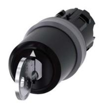
Key-operated switch IKON, 22 mm, round, plastic with metal front ring, lock number 360012K1, with 2 keys, 3 switch positions I-O-II, latching, actuating angle  $2x45^{\circ}$ , 10:30h/12h/13:30h, key removal O, with laser labeling, lower case
