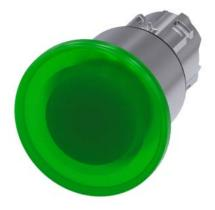
Illuminated mushroom pushbutton, 22 mm, round, metal, shiny, green, 40 mm, 3 switch positions, latches after pushing in, unlatches by pull-to-unlatch mechanism to center position, after pulling out the button Retraction to center position, Z=50-unit packaging
