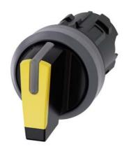
Selector switch, illuminable, 22 mm, round, plastic with metal front ring, yellow, selector switch, short, 3 switch positions I-O<II, left latching, right momentary contact type, actuating angle 2x45°, 10:30h/12h/13:30h, with laser labeling, lower case
