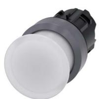
Illuminated mushroom pushbutton, 22 mm, round, plastic with metal front ring, white, 30 mm, momentary contact type, with laser labeling, upper case
