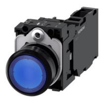
Illuminated pushbutton, 22 mm, round, plastic, blue, pushbutton, flat, momentary contact type, with holder, 1 NO+1 NC, LED module with integrated LED 24 V AC/DC, screw terminal, with laser labeling, symbol number according to, ISO 7000 or IEC 60417
