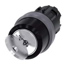
RONIS key-operated switch, 22 mm, round, plastic with metal front ring, lock number SB30, with 2 keys, 2 switch positions O-I, latching, actuating angle 90°, 10:30h/13:30h, key removal O, possible special locks: SB31, 421, 455, with laser labeling, upper case and lower case, always upper case at beginning of line
