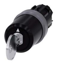
Key-operated switch BKS, 22 mm, round, plastic with metal front ring, special lock, with 2 keys, 3 switch positions I-O<II, latching on the left, momentary contact type on the right, actuating angle 2x45°, 10:30h/12h/13:30h, key removal I, Note: BKS locking systems E1 - E25 supplied without key
