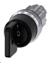
Key-operated switch O.M.R, 22 mm, round, metal, shiny, lock number 73034, black, with 2 keys, 3 switch positions I>O<II, momentary contact on the left, latching on the right, actuating angle 2x45°, 10:30h/12h/13:30h, Key removal II, with laser labeling, upper case and lower case, always upper case at the beginning of the word
