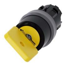
Key-operated switch O.M.R, 22 mm, round, plastic with metal front ring, lock number 73033, yellow, with 2 keys, 2 switch positions O-I, latching, actuating angle 90°, 10:30h/13:30h, key removal O, with laser labeling, upper case and lower case, always upper case at beginning of line
