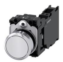
Pushbutton, 22 mm, round, metal, shiny, white, pushbutton, flat, momentary contact type, with holder, 1 NO+1 NC, spring-type terminal, with laser labeling, upper case
