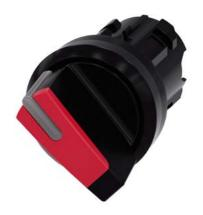
Selector switch, illuminable, 22 mm, round, plastic, red, selector switch, short, 2 switch positions O<I, momentary contact type, Actuating angle 45°, 10:30h/12h, with laser labeling, upper case and lower case, always upper case at the beginning of the word
