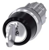
RONIS key-operated switch, 22 mm, round, metal, shiny, lock number SB30, with 2 keys, 3 switch positions I>O<II, momentary contact on the left, latching on the right, actuating angle 2x45°, 10:30h/12h/13:30h, Key removal O+II, possible special locks: SB31, 421, 455, with laser labeling, upper case and lower case, always upper case at the beginning of the word
