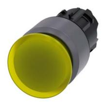
Illuminated mushroom pushbutton, 22 mm, round, plastic with metal front ring, yellow, 30 mm, latching, pull-to-unlatch mechanism, with laser labeling, symbol number according to, ISO 7000 or IEC 60417
