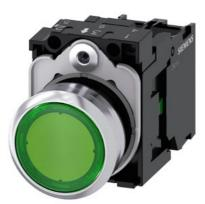
Illuminated pushbutton, 22 mm, round, metal, shiny, green, pushbutton, flat, momentary contact type, with holder, 1NO, LED module with integrated LED 24 V AC/DC, screw terminal, with laser labeling, lower case
