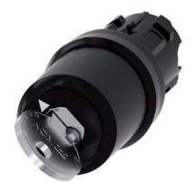
Key-operated switch IKON, 22 mm, round, plastic, lock number 360012K1, with 2 keys, 2 switch positions O<I, momentary contact type, Actuating angle 45°, 10:30h/12h, key removal O, with laser labeling, upper case and lower case, always upper case at beginning of line
