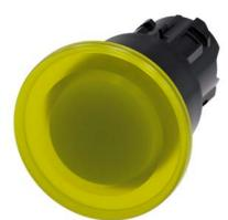
Illuminated mushroom pushbutton, 22 mm, round, plastic, yellow, 40mm, latching, pull-to-unlatch mechanism, with laser labeling, symbol number according to, ISO 7000 or IEC 60417
