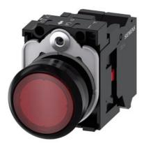
Illuminated pushbutton, 22 mm, round, plastic, red, pushbutton, flat, momentary contact type, with holder, 1NC, LED module with integrated LED 230 V AC, spring-type terminal, with laser labeling, inscription or symbol Customer-specific selection with SIRIUS ACT configurator (CIN)
