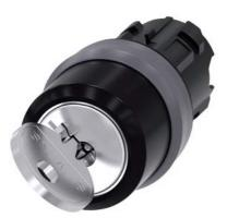
RONIS key-operated switch, 22 mm, round, plastic with metal front ring, lock number SB30, with 2 keys, 2 switch positions O-I, latching, actuating angle 90°, 10:30h/13:30h, key removal I, possible special locks: SB31, 421, 455, with laser labeling, lower case
