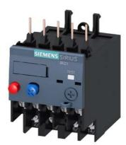
Overload relay 0.14...0.20 A Thermal For motor protection Size S00, Class 10 Contactor mounting Main circuit: Ring cable lug Auxiliary circuit: ring cable lug Manual-Automatic-Reset
